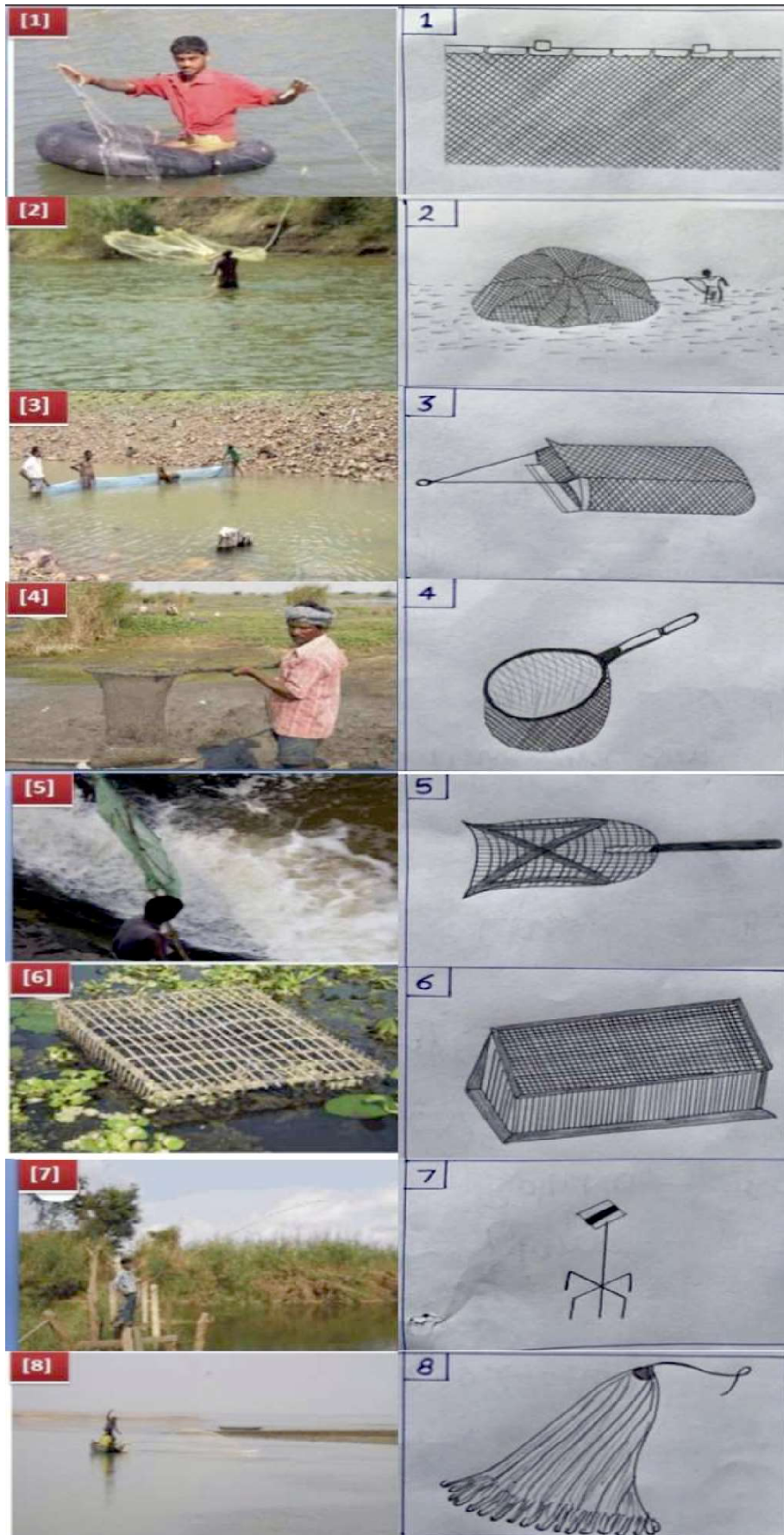
Fig, 1 : A view on different types of gear (1) Gill net, (2) Cast net, (3) Dragged net, (4) Dip net, (5) Hand net, (6) Trap, (7) Hooks (8) Hanging rope. Adapted and modified.
